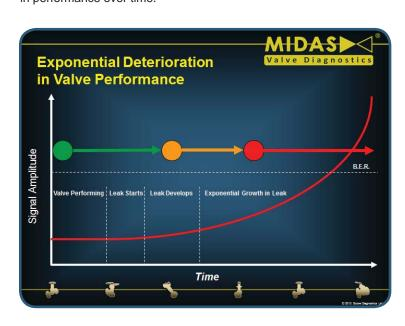
Given that we know this, it is possible to use Acoustic Emissions (AE) technology, for example, for quick and easy leak detection.
